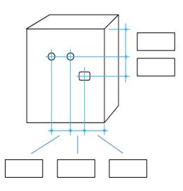
Note that the positions of these holes are reversed in relation to the view of the wall, because you are looking at the back of the cabinet.
